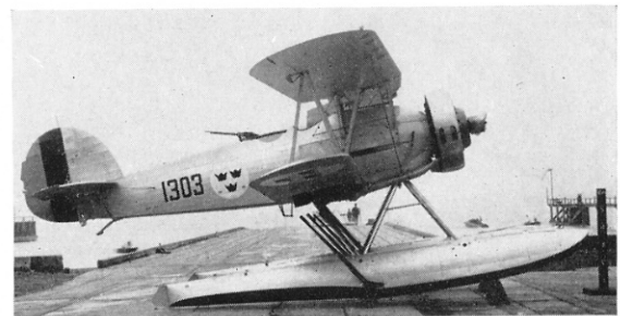
Third Swedish Hart, 1303, with Short S.51 floats at Felixstowe. This was used as a pattern aircraft for Swedish Ospreys which subsequently served aboard the aircraft-equipped cruiser Gottland.
