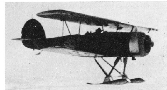
Only known air photo of a ski-equipped Swedish Hart; this aircraft is powered by a long-chord-cowled Pegasus engine. (Photo: Zeitschrift fuer Flugtechnik und Motorluftschiffahrt)
